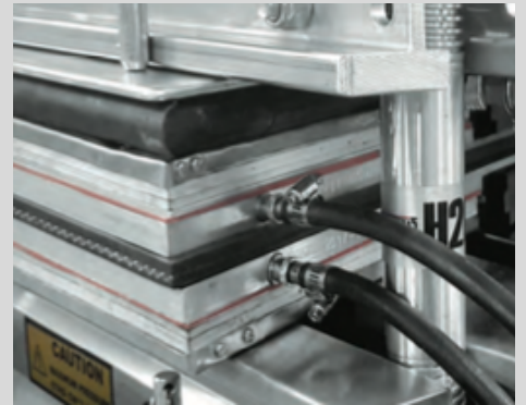
Rubber pressure bag for even distribution
